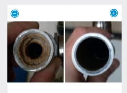
**Pipes with AquaKat**Conductor condition after three months of operation without and with AquaKat.
